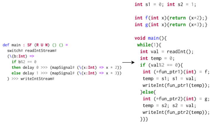
Figure 11: Code generation for switch#
